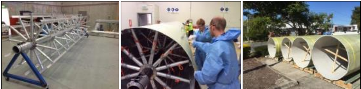
Fig. 4. Construction of StifPipe® at QuakeWrap facilities in Brisbane, Australia
