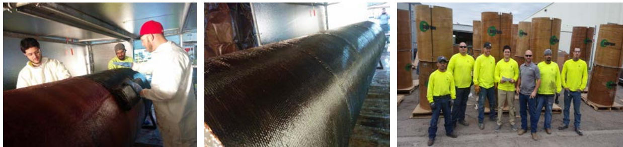
Fig. 6. Manufacturing of PM carbon FRP pipe in Tucson and the finished pipe segments prior to shipment to Puerto Rico
