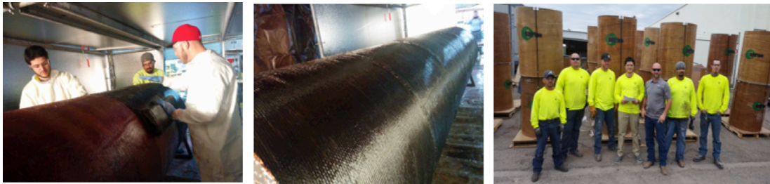
Fig. 7. Manufacturing of PM carbon FRP pipe in Tucson and the finished pipe segments prior to shipment to Puerto Rico
