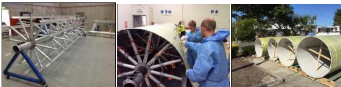
Fig. 3. Construction of SC pipe at QuakeWrap facilities in Brisbane, Australia
