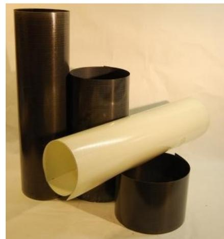
Figure 2. New laminates: carbon (black) and glass (white).
