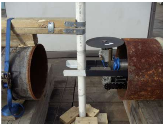
Figure 14. Simulated drip pot with standpipe laboratory test set-up.
