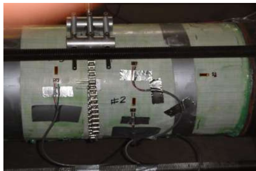
Figure 9. Typical Instrumented test specimen
