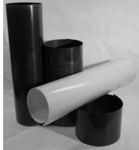
Figure 3. Samples of PipeMedic™ laminates constructed with carbon and glass fabric.
