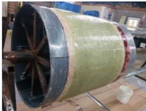
Figure 4. StifPipe® sample being made on a mandrel by applying resin saturated glass, carbon, and 3D fabric layers.
