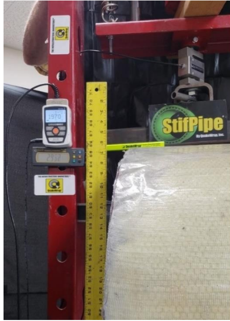
Figure 7. A 36-inch StifPipe® at 1,970 lb. of parallel plate load with no apparent sign of a failure.
