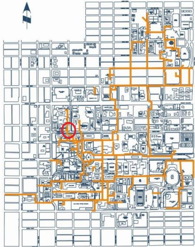
Fig. 1. The network of 6 ½ miles of utility tunnels under the campus of the University of Arizona; the project site is shown with a red circle.
