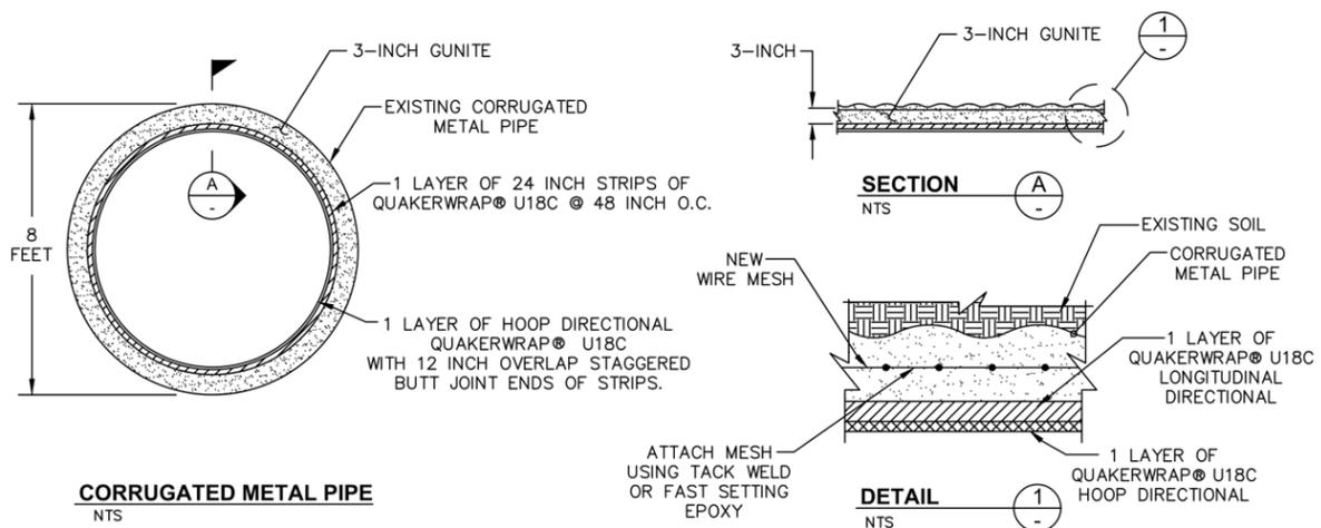
Fig. 4. Design of the retrofit system for the corrugated metal pipe tunnel.
