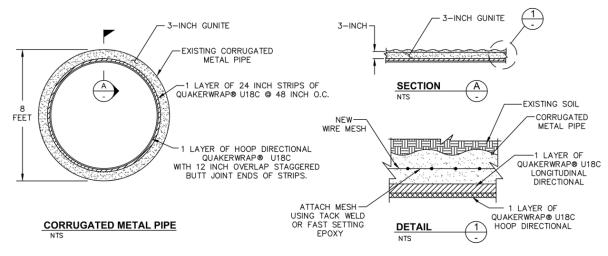
Fig. 4. Design of the retrofit system for the corrugated metal pipe tunnel.
