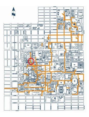
Fig. 1. The network of 6  $\frac{1}{2}$  miles of utility tunnels under the campus of the University of Arizona; the project site is shown with a red circle.
